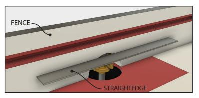
Use a straightedge to set the fence flush with the router bit's bearing. Place the straightedge against the bearing and adjust the fence until it's flush. Lock the fence into position.
