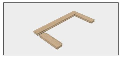
Apply glue to the tenons on both rails, assemble the door and clamp. Allow the glue to set completely before removing it from the clamps (at least 30 minutes).
