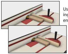
Use a miter gage or coping sled to cope both ends of the rails.
