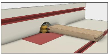
With this bit, it's not necessary to reposition the fence for the profile cut, but you will need to adjust the bit height. Place one of the rails you just routed face down on the router table. Align the bit with the cope cut in one end of the rail.
