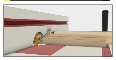
To prevent excessive tear-out on one end of each rail, make the cope cuts before the inside edge profile cuts. Insert the bit in the router table and adjust the height to produce a small flat spot of 1/16" to 1/8" near the top face.
